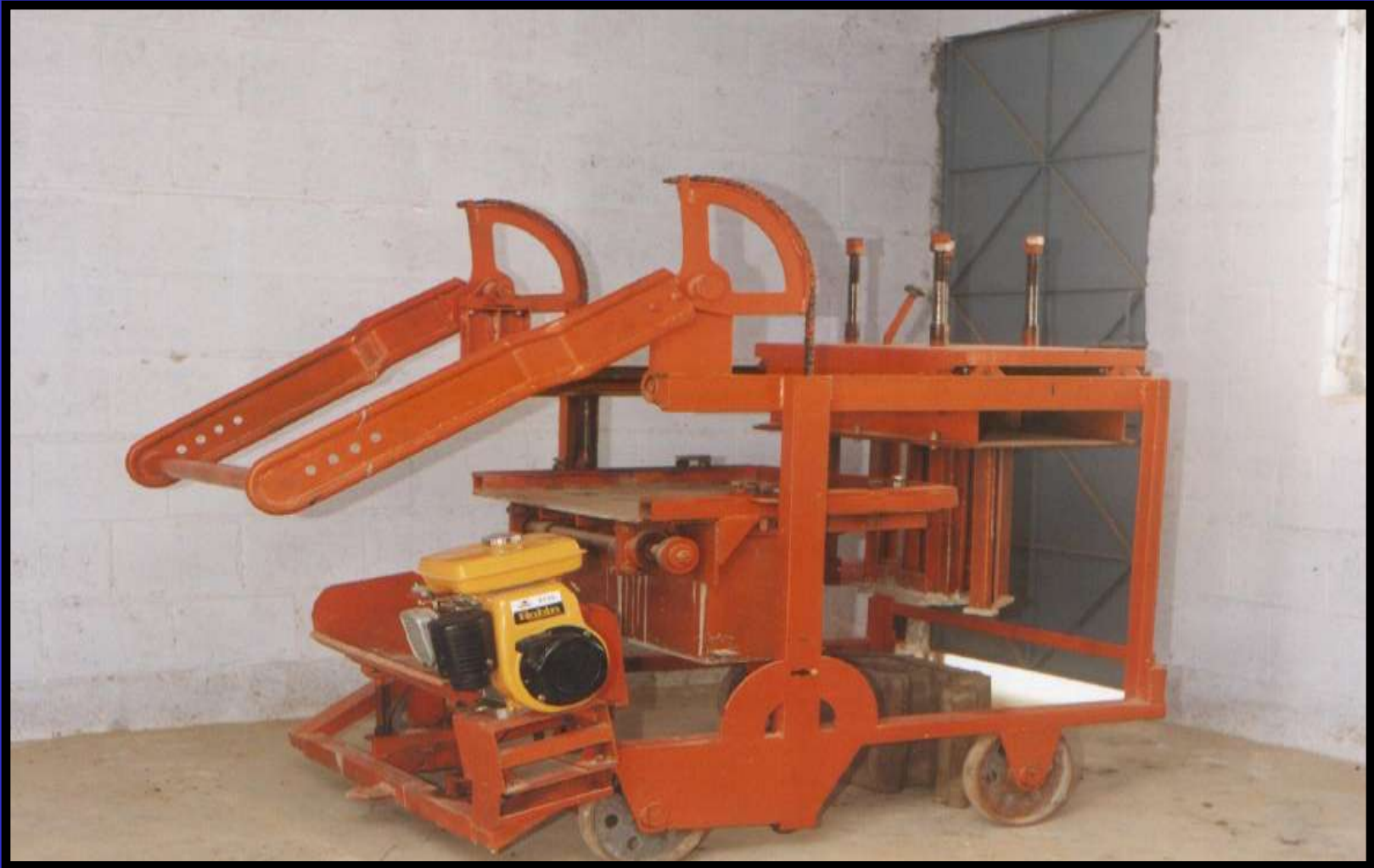
Machine Developed for Casting Pre-cast Concrete Blocks For Water Course Lining
