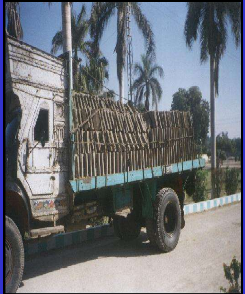
Transportation of Lining Unit from CWHR to Site
